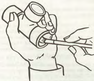
Figure 4-8 Flux all the cups on a fitting as soon as they are clean and assemble.
