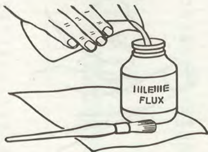
Figure 4-9 Add water as necessary to keep flux at the right consistency. Don't let the brush get dirty.
