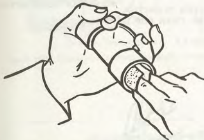
Figure 4-7 With abrasives, clean out the cup and chamfer of each fitting outlet.
