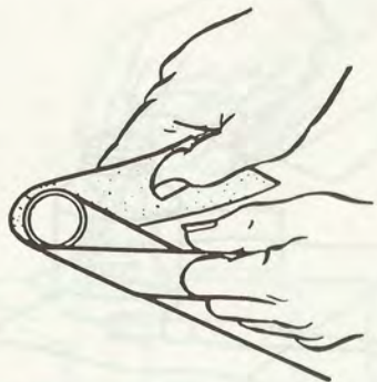
Figure 4-4 Use abrasives to get scale and dirt off the end of the pipe.
