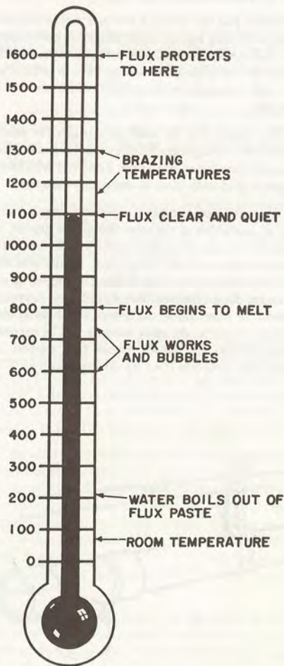
Figure 3-7 Here is how flux behaves as a temperature indicator.
