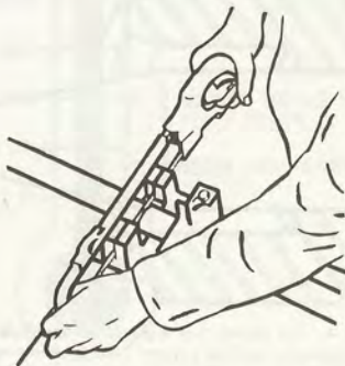
Figure 3-2 A square-end sawing vise holds the pipe and guides your hack saw for a square cut.
